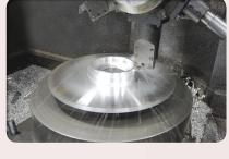
Precise machining for flange and barrel by vertical CNC lathe machines.
