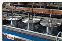
Hard-Anodizing treatment for protection against corrosion and damage.
