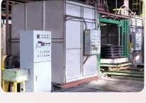
Ouenching & Tempering(T-6) of flanges and barrels using the newest heat treatment furnace.
